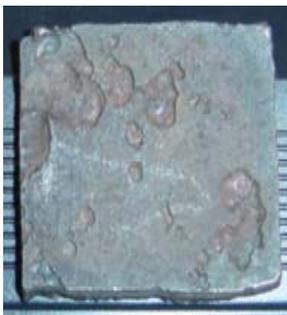
**Pin Hole Corrosion as a result of anaerobic bacterial activity**
